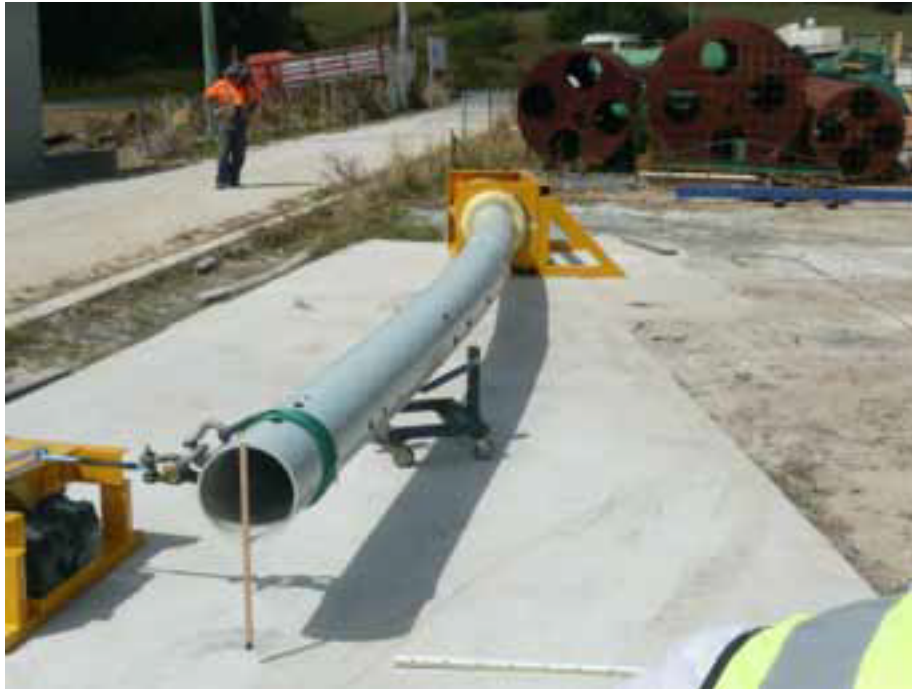
Fig 4. – Pole at 25 kN Tip Load
