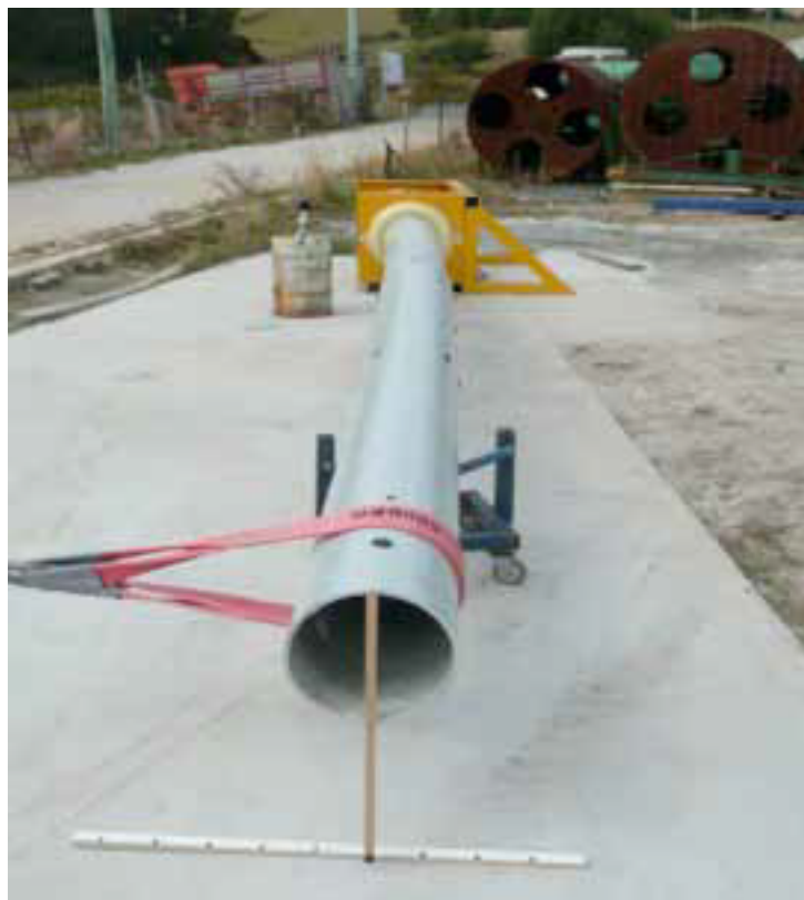
Fig 3. – Pole at 8 kN
